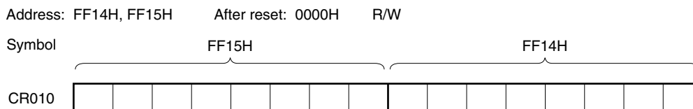
Figure 6-4. Format of 16-Bit Timer Capture/Compare Register 010 (CR010)
