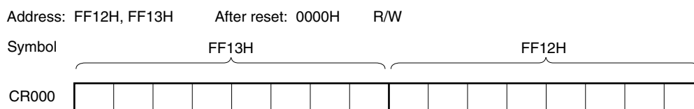
Figure 6-3. Format of 16-Bit Timer Capture/Compare Register 000 (CR000)
